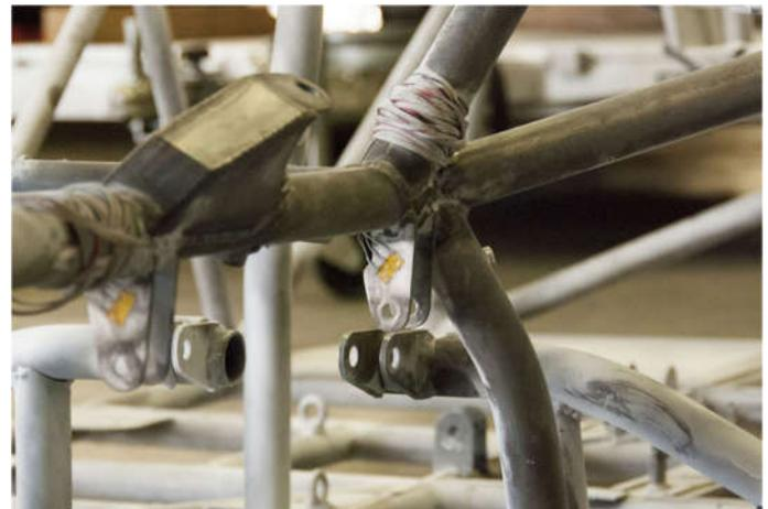
**Figure 4. Strain gauge sensors as installed to suspension arm of initial chassis design**
